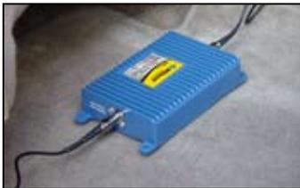
Run the cable from the Outside Antenna and attach it to the connector labeled "Outside Antenna" on the Signal Booster.
