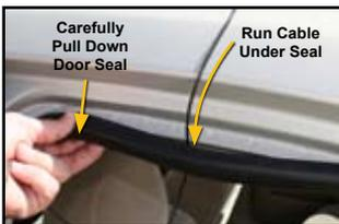
For a more professional looking installation, run the antenna cable under the door seal. The antenna cable is small enough to easily tuck under the door seal or plastic molding. Carefully pull down the door seal. Run the cable through the seal and push the seal back into place. This prevents constant wear and tear on the cable as the door opens and closes.
