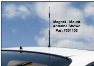
Separation of the Inside and Outside Antennas is very important. The metal roof of the vehicle acts as a barrier and helps shield the two antennas from each other, preventing oscillation (feedback).
