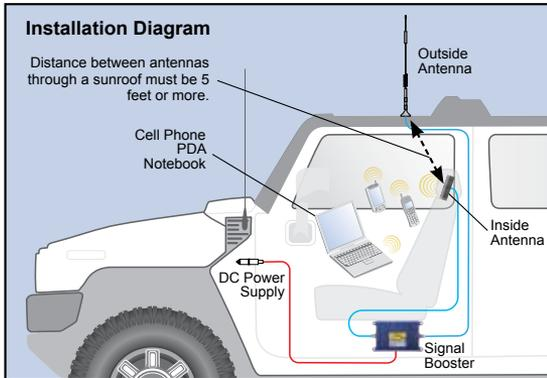
**Warning:** In a wireless installation, do not plug the Signal Booster directly into the cell phone and/or data card using an antenna adapter. It may damage the Signal Booster, cell phone and/or data card.
